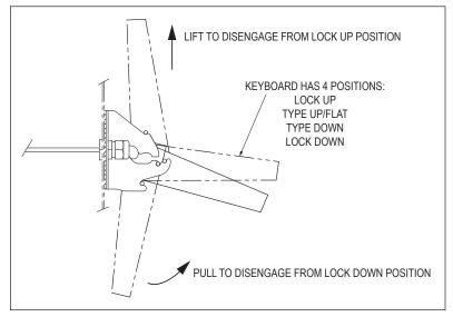
FIGURE 10 – SIDE VIEW SHOWING 4 POSITIONS
