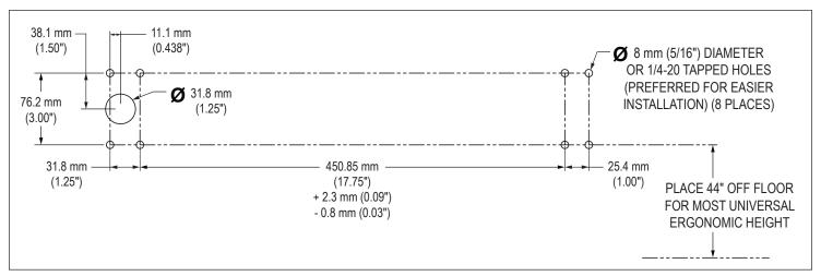
FIGURE 1 - PANEL MOUNTING PATTERN
