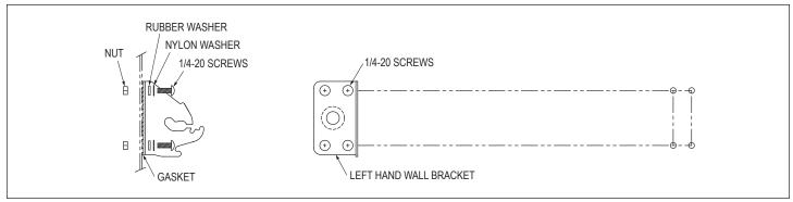
FIGURE 2 - SIDE VIEW AND FRONT VIEW OF LEFT HAND WALL BRACKET
