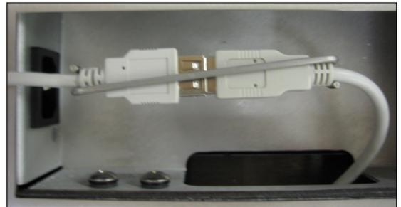
12. Insert the KVM Remote Module into the opening of the rear panel by sliding the right hand locking tabs in all the way to the right.
