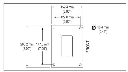
FIGURE 1 - PEDESTAL BASE PLATE
